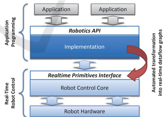
Figure 1: Robot application are programmed against the *Robotics API*. High-level commands specified using the *Robotics API* are automatically transformed into dataflow graphs at runtime and executed with real-time guarantees.
