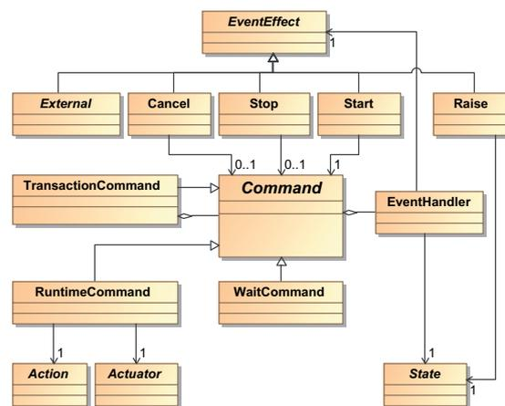
Figure 3: Commands in the Robotics API.
