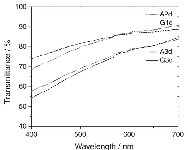
**Figure 2.** Optical transmission spectra of pure bacterial cellulose (BC) membranes.
