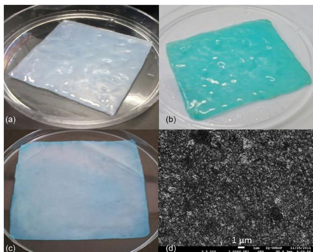
**Figure 3.** Photographs of pure bacterial cellulose (BC) wet membrane (a); BC- chloroaluminum phthalocyanine (CIAIPc) wet (b); dried BC-CIAIPc membrane (c); and scanning electron microscope (SEM) image of BC-CIAIPc (d).
