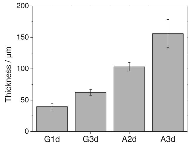
**Figure 1.** Thickness of pure bacterial cellulose (BC) membranes.
