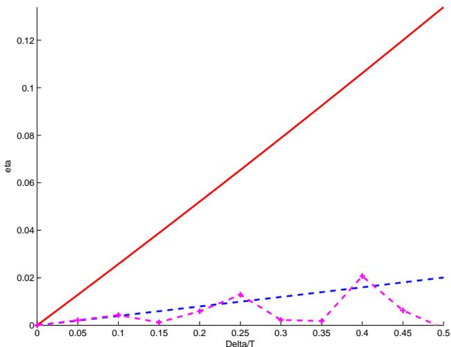
Fig. 3. *Top curve.* Upper bound on  $\eta$  over all initial states (solid red). *Bottom two curves.* Heuristic lower bound on  $\eta$  (dashed blue) and Monte Carlo simulation with identical initial state (magenta). Sampling period  $T = 0.01$  secs.
