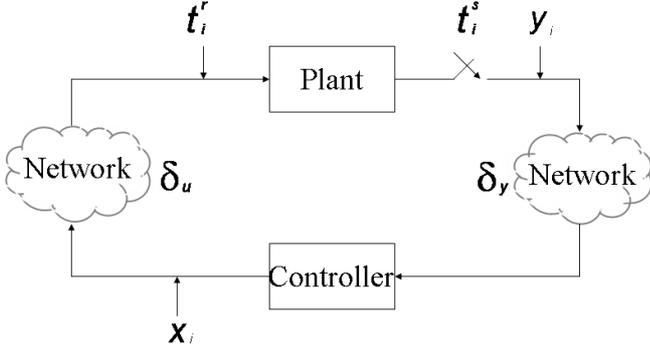
Fig. 1. Plant and controller with network delays.
