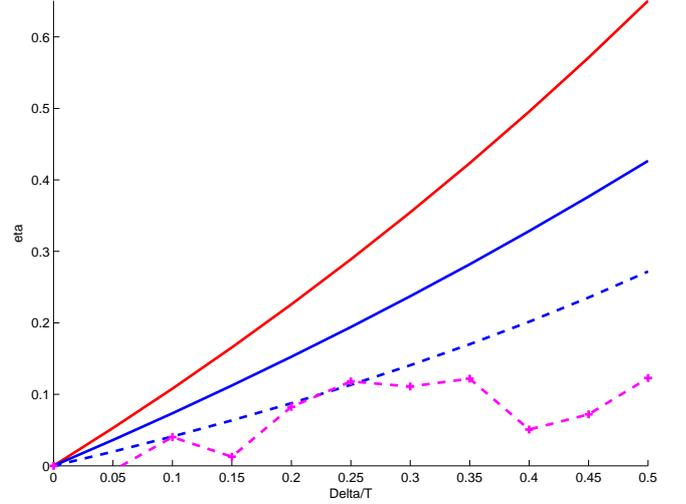
Fig. 2. Top two curves. Upper bound on  $\eta$  over all initial states (solid red) and for a specific initial state (solid blue). Bottom two curves. Heuristic lower bound on  $\eta$  (dashed blue) and Monte Carlo simulation with identical initial state (magenta). Sampling period  $T = 0.1$  secs.
