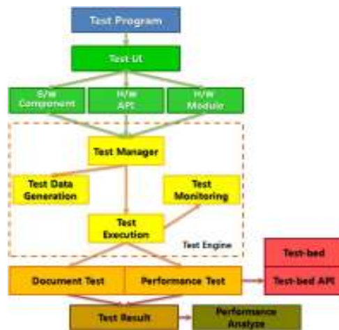
Figure 7. Block Diagram of Overall Testing System
