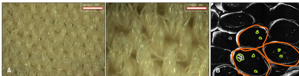
**Fig. 1.** Optical and electron microscopic structures of the anion textile. (A)  $\times 100$ ,  $\times 300$ , (B)  $\times 2,000$ . The anion textile fibers are regular and rounded without stubby ends, resulting in a smooth feeling overall. The polyester filaments (orange circle) contain nano-sized fine-crusted tourmaline powder (green circle).
