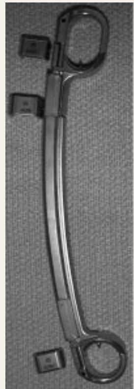
Figure 4. Vertical Expansion Prosthetic Titanium Rib (VEPTR) Device consisting of extensible titanium rod/sleeve constructs of varying length. Two radii of curvature are available for different applications to conform to or modify the surface contour of the thoracic cage. Ring-like capturing devices (rib cradle and end cap) on each end are placed around one or two healthy ribs above and below the expansion thoracostomies for chest expansion. The basic configuration consists of superior cradle, cradle end halves, cradle locks or rib sleeve, inferior cradle, or lumbar extension, and distraction locks. The inferior cradle may be replaced with a lumbar extension rod/hook combination to act as a spinal distraction device (hybrid device). With growth, the rod/sleeve is extended (distracted) through a small incision. When maximum length is achieved, the rod/sleeve is replaced with a longer construct.
