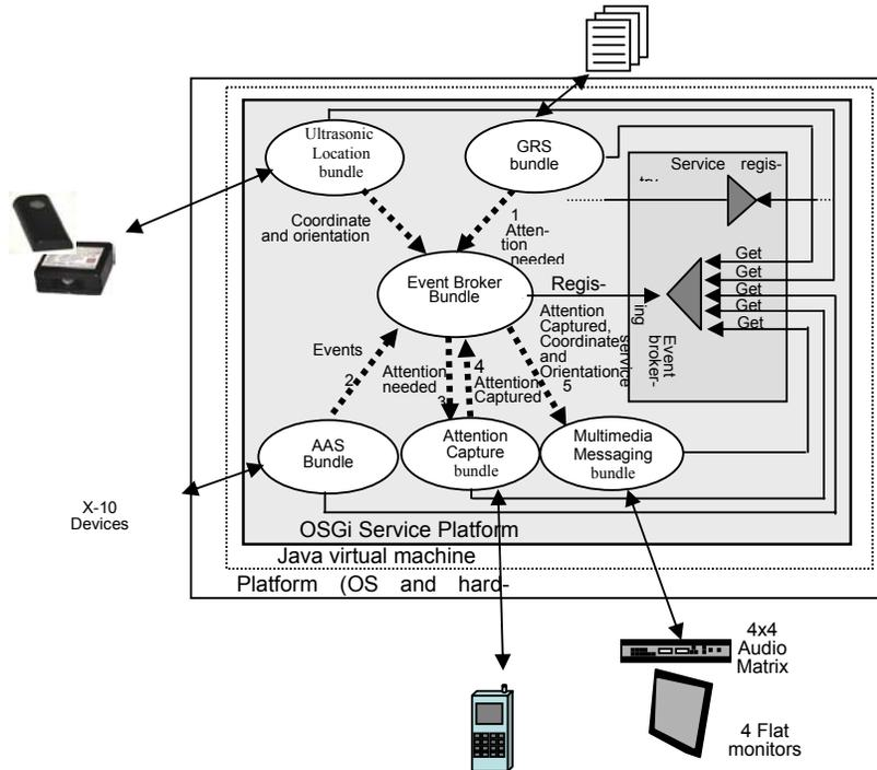
**Figure 2. Applications as bundles on the OSGi framework.**
