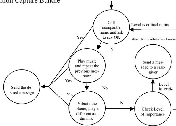
Fig. 3. Transition diagram for cuing a blind person.
