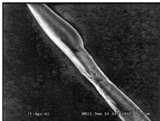
Figure 3. Cold field emission scanning electron microscope (CFE-SEM) micrograph of a damaged Heterorhabditis bacteriophora after flow through the contraction at a volumetric flow rate of 24.78 \text{cm}^3/\text{s} , which shows a region of deformation (i.e., necking) near the center of the nematode body.
