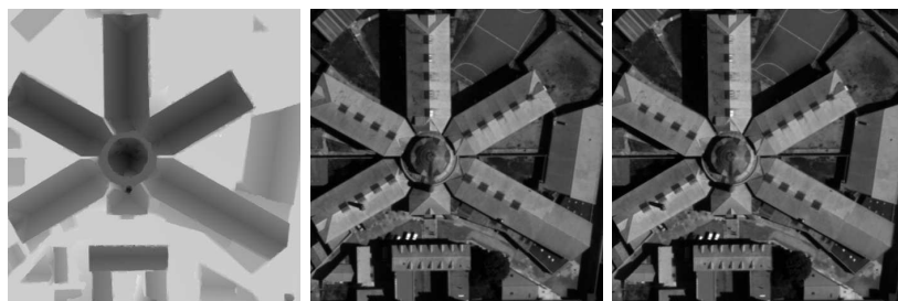
Figure 7: Synthetic image pair. Left: the disparity ground truth. The background has uniform disparity while the building simulates the slope of a roof. Center and right: image pair.
