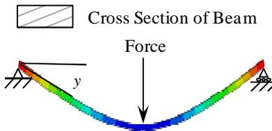
Fig. 6 Schematic of the simply supported beam.
