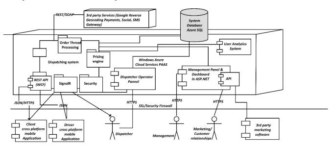
Figure 6. General Dispatching System Architecture.
