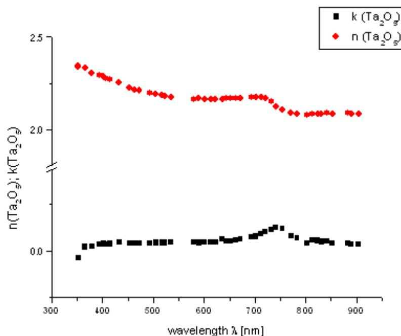
**Figure 1.** Refractive index  $n$  and extinction coefficient  $k$  of a thin  $\text{Ta}_2\text{O}_5$  layer on glass ( $n = 1.52$ ) versus wavelength (light source: Xe arc lamp with corresponding interference filters); measurements performed at an angle of incidence of  $50^\circ$  by means of spectroscopic ellipsometry (EP<sup>3</sup>, Nanofilm Technologie GmbH, Göttingen, Germany).
