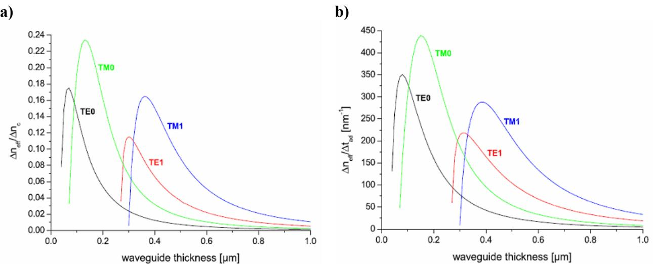
**Figure 4.** Theoretical sensitivities of a waveguide to a) cover refractive index changes and b) surface adlayer changes versus waveguide thickness. Parameters for calculation:  $n_s = 1.52$ ,  $n_w = 2.1$ ,  $n_c = 1.333$  and  $\lambda = 675$  nm. From [21].
