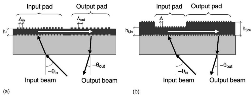
**Figure 9.** (a) Cut through dual period sensor chip. (b) Cut through thickness-modulated sensor chip. From [46], Copyright Elsevier (2003).
