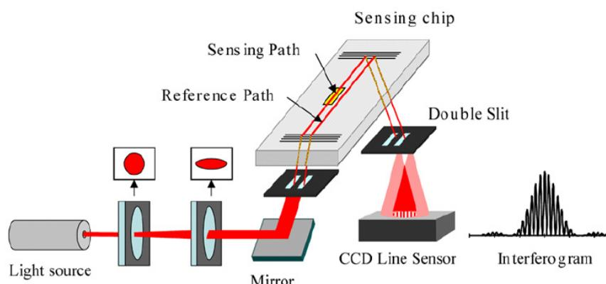
**Figure 10.** Young interferometer as described in [21]. Light from a light source is coupled into the waveguide sensor chip by a grating after being split in two beams by a double slit. The two beams are guided separately down the waveguide, forming sensing and reference path, and coupled out by a second grating. The interference pattern is recorded behind another double slit by a CCD line sensor.
