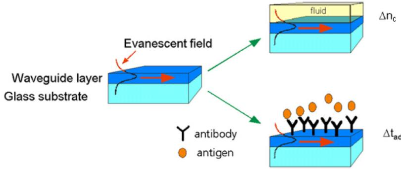
**Figure 3.** The principle of evanescent field sensing. A waveguide layer on a substrate is guiding a light mode with phase velocity  $v_1$ . A change in the effective refractive index and thus a decrease in the phase velocity  $v_2 < v_1$  is caused by either a change in the cover refractive index  $\Delta n_c$  or a change in the adlayer thickness  $\Delta t_{ad}$  due to molecule adsorption, e.g. binding of an antigen to a capture antibody. From [21].
