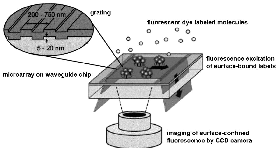
**Figure 12.** Detection principle of evanescent field fluorescence on planar waveguides (principle of ZeptoREADER): excitation light is coupled into a thin-film waveguide; surface confined fluorescence of bound labeled molecules is detected by a CCD camera. Adapted from [2, 19]
