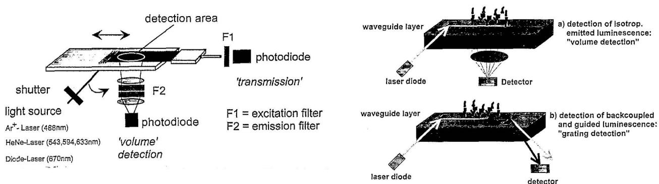
**Figure 11.** left: Schematic optical set-up used for first model-assays for 'volume detection', interference filters were used for selection of the excitation or emission light and photodiodes or photomultiplier for signal detection; right: comparison of set-ups for volume detection and detection of backcoupled and guided luminescence light, using a second outcoupling grating where different wavelength can be discriminated by the outcoupling angle. From [31], Copyright Elsevier (1997).
