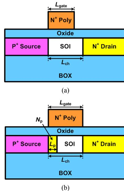
**Fig. 5.** Device structures of (a) short-gate TFET and (b) PNP MOSFET.
