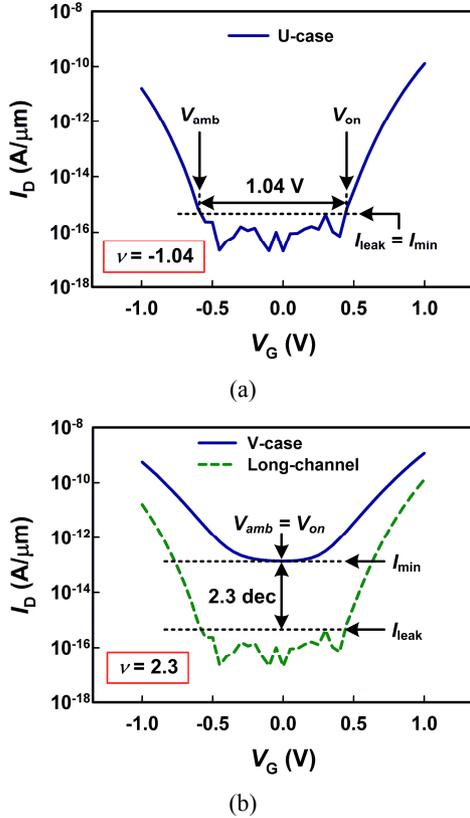
**Fig. 4.** The extraction method of  $\nu$  for (a) U-case and (b) V-case.
