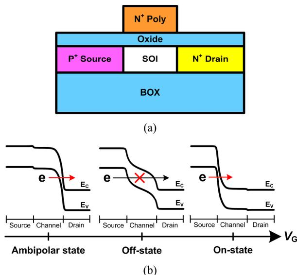
**Fig. 1.** (a) Conventional n-channel SOI TFET structure, (b) Band diagrams of the TFET in ambipolar, off- and on-state. As  $V_G$  increases, the TFET experiences ambipolar, off- and on-state sequentially.
