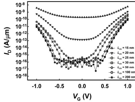
**Fig. 3.**  $I_D$ - $V_G$  curves with  $L_{ch}$  ranging from 15 to 500 nm. As  $L_{ch}$  decreases, BTBT current increases and also off-current.
