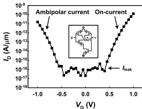
**Fig. 2.** Simulated  $I_D$ - $V_G$  curve of an SOI TFET.  $I_D$  consists of three components: on-current,  $I_{leak}$  and ambipolar current. The inserted figure shows a 2-input NAND gate. Squarred bracket indicates the location of the tunneling junction.
