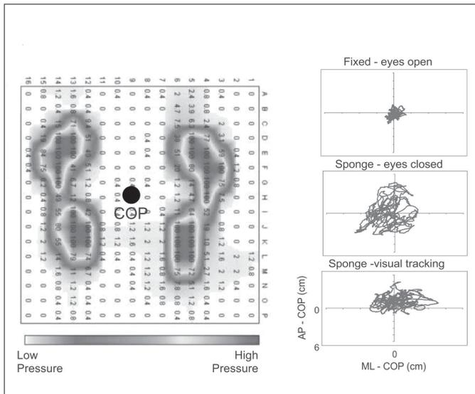
**Figure 2.** Presents a snapshot of the pressure mat in standing and example XY-plots of ML-AP COP excursions for different test conditions on fixed and sponge surfaces.
