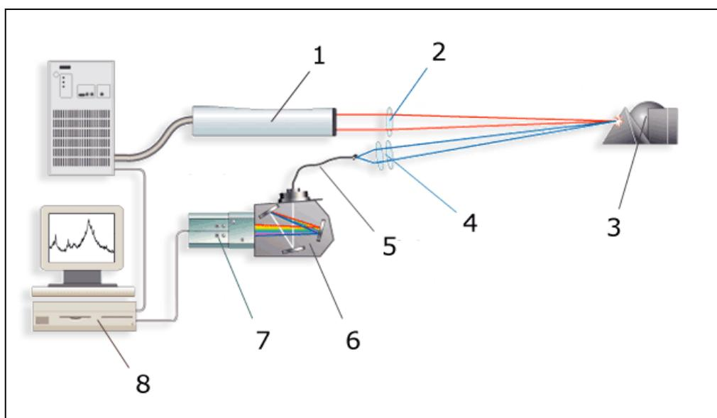
**Figure 1.** The LIBS experimental setup. 1 – Nd:YAG ablation laser, 2 – focusing optics, 3 – the analyzed sample, 4 – collecting optics, 5 – optical fiber, 6 – monochromator, 7 – ICCD camera, 8 – personal computer.
