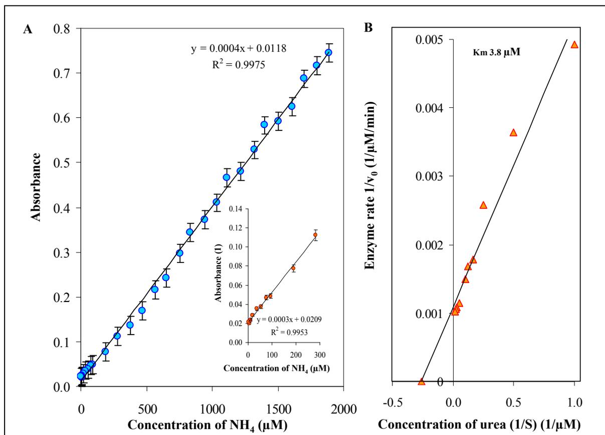
**Figure 10.** Spectrometric automated analysis of urease activity. The dependence of total amount of released ammonia on height of the obtained signal (A). Enzyme kinetic of soybean urease (B).
