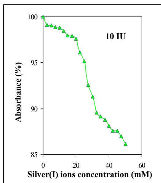
**Figure 12.** The changes of activity of commercially available urease in the presence of silver(I) ions.
