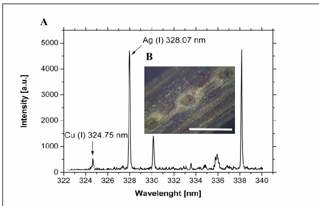
**Figure 6.** The typical LIBS spectrum with the 328.07 nm Ag(I) and 324.75 nm Cu(I) lines used in the analysis (A) together with the image of three ablation craters (B). The bar on B has a length of 500  $\mu$ m.
