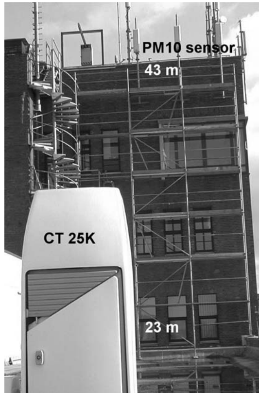
Fig. 4 Measurement set-up for ceilometer aerosol concentration measurements, PM10 and PM2.5 inlet probes level is 20 m above the ceilometer
