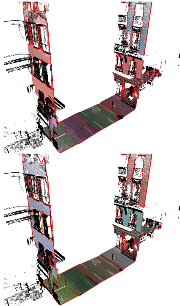
Figure 6. Results of SSP-RANSAC for varying alpha shape radius: top  $\alpha = 2$  cm, bottom  $\alpha = 20$  cm.
