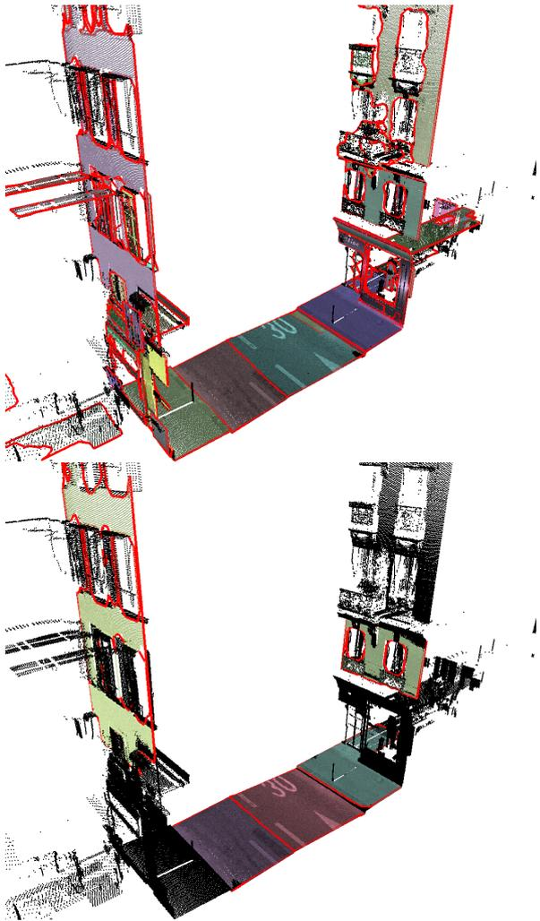
Figure 5. Results of SSP-RANSAC for varying minimum patch size: top  $n_{\min} = 500$ , bottom  $n_{\min} = 10\,000$ .
