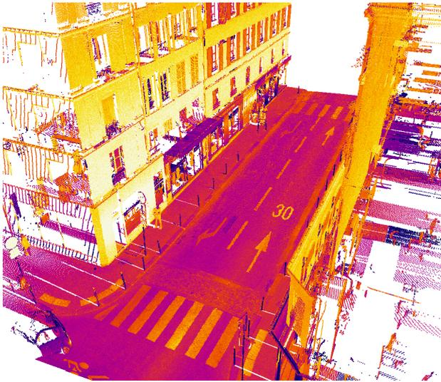
Figure 1. A view of the Mobile Laser Scan (MLS) used in this study, colored with reflectance.
