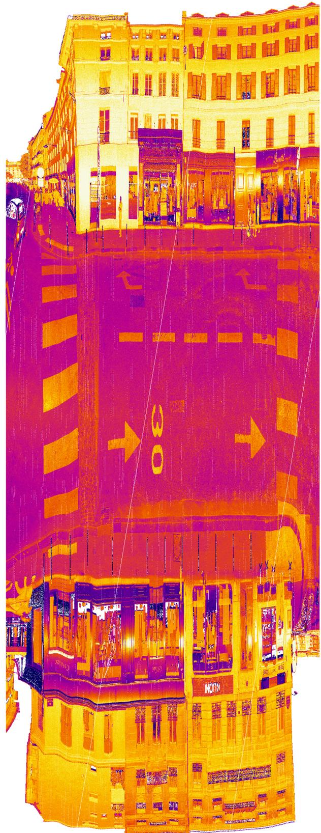
Figure 2. A view of the same Mobile Laser Scan (MLS) colored with reflectance in sensor space (horizontally: time, vertically:  $\theta$ ). For multiple echoes, the last is used. For no returns, we keep the white background color.
