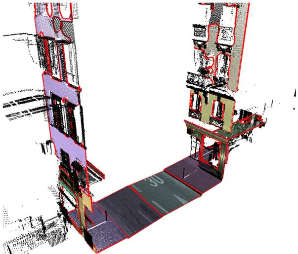
Figure 3. A view of a result of our sensor space enhanced polygonal RANSAC with a reference set of parameters. Point attributed to a planar patch have a different hue for each patch, unattributed points are in black. The extracted planar polygonal outlines are in red.
