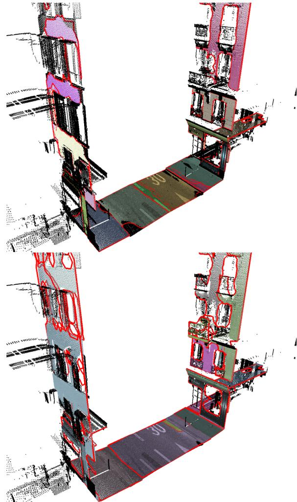
Figure 4. Results of SSP-RANSAC for varying inlier threshold: top  $d_{in} = 1$  cm, bottom  $d_{in} = 10$  cm.
