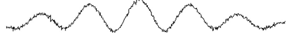
Fig. 12. Double-slit interference with a low-pressure Na light source. The graph and image grayscale is 0–500 counts.
