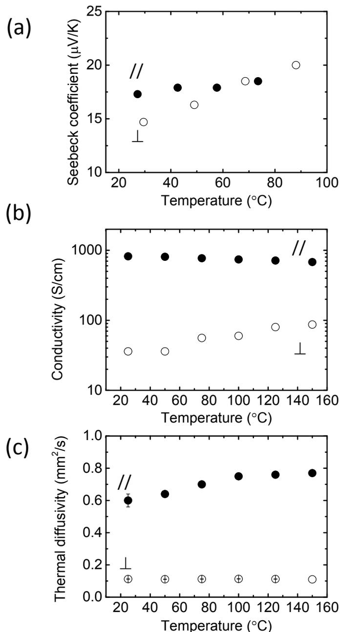
**Figure 8.** (a) Seebeck coefficient, (b) electrical conductivity, and (c) thermal diffusivity of the PEDOT/PSS films in the in-plane (closed circles) and through-plane (open circles) directions, plotted as a function of temperature. Reproduced with permission from [37]. Copyright 2014 American Chemical Society.
