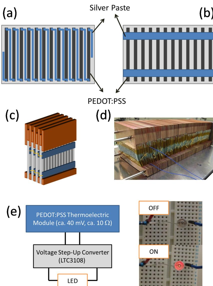
**Figure 9.** Schematic representation of the (a) series and (b) parallel PEDOT:PSS array. (c) Schematic and (d) photograph of the PEDOT:PSS modules sandwiched between copper plates. (e) Schematic of the circuit for powering an LED and photograph of the LED driven by the PEDOT:PSS thermoelectric module. Reproduced with permission from [68]. Copyright 2014 The Royal Society of Chemistry.
