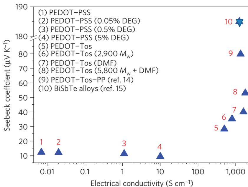
**Figure 5.** Seebeck coefficient *versus* electrical conductivity of various PEDOT derivatives including pristine PEDOT/PSS and diethylene glycol (DEG)-containing samples, chemically polymerized PEDOT/Tos as well as three VPP PEDOT/Tos samples with triblock copolymers PEG-PPG-PEG with different M<sub>w</sub>. Reproduced with permission from [48]. Copyright 2014 Nature Publishing Group. (PEG = polyethylene glycol, PPG = polypropylene glycol).
