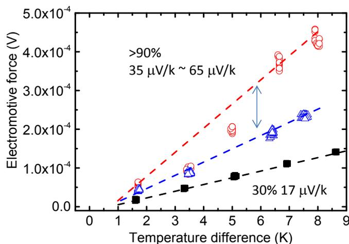
**Figure 7.** Seebeck coefficient measurements of PEDOT:PSS films at different humidity levels. Closed circles represent Seebeck coefficient measurements at a humidity of 30% and open circles represent Seebeck coefficient measurements at a humidity larger than 90%. Reproduced with permission from [31]. Copyright 2014 Japan Society of Applied Physics.
