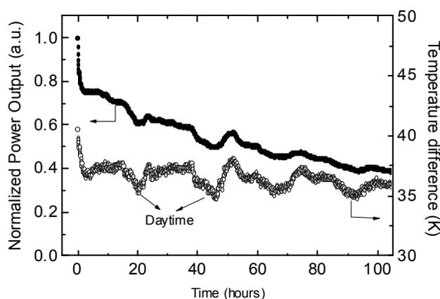
**Figure 10.** Power output of module and temperature difference as a function of the working time. Reproduced with permission from [68]. Copyright 2014 The Royal Society of Chemistry.
