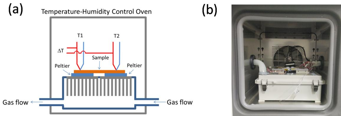
**Figure 3.** (a) Schematic and (b) photographic images of the Seebeck measurement setup in high-humidity conditions. Reproduced with permission from [31]. Copyright 2014 Japan Society of Applied Physics.
