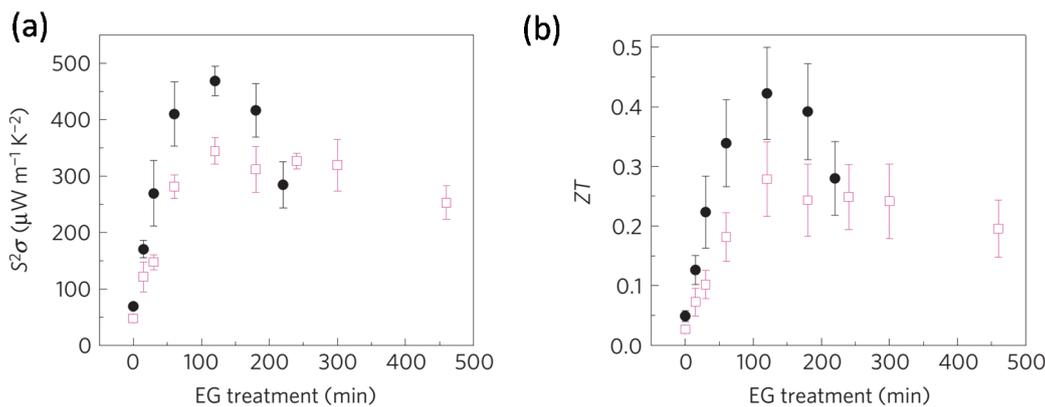
**Figure 6.** (a) Thermoelectric power factors and (b) thermoelectric figure-of-merit at 297 K in EG-mixed (open squares) and dimethyl sulfoxide (DMSO)-mixed (closed circles) PEDOT:PSS measured during the EG treatment (dedoping) process. Reproduced with permission from [49]. Copyright 2013 Nature Publishing Group.
