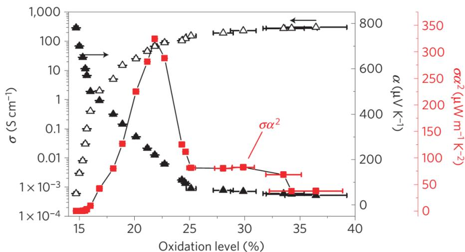
**Figure 4.** Seebeck coefficient (filled triangles), electrical conductivity (open triangles) and corresponding power factor (red squares) *versus* oxidation level of the PEDOT/tos films. Reproduced with permission from [46]. Copyright 2011 Nature Publishing Group.
