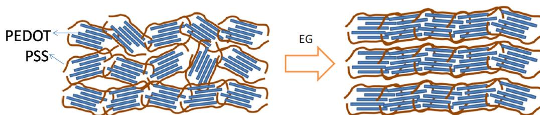
**Figure 2.** Morphological change in the PEDOT:PSS films caused by the addition of ethylene glycol (EG). Reproduced with permission from [22]. Copyright 2013 Wiley–VCH Verlag GmbH & Co.
