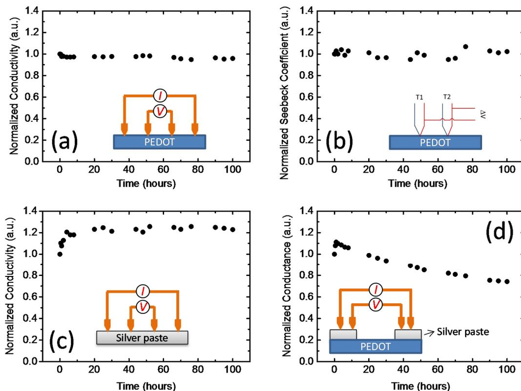
**Figure 11.** (a) Electrical conductivity and (b) Seebeck coefficient of PEDOT:PSS, and (c) electrical conductivity of silver paste and (d) conductance of silver paste/PEDOT:PSS/silver paste as a function of time at 80 °C. Reproduced with permission from [68]. Copyright 2014 The Royal Society of Chemistry.
