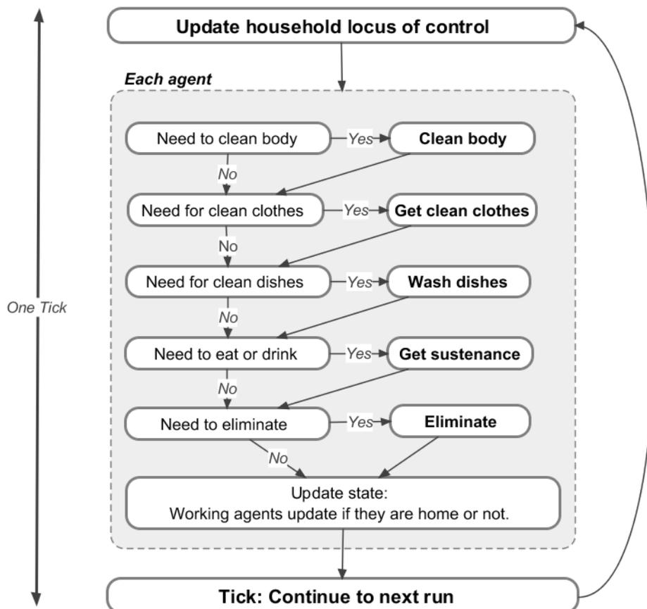
**Figure 4.** Graphical representation of the agent decision-making process in the model to execute each of the water use habits: clean body, get clean clothes, wash dishes, get sustenance and eliminate. An agent perceives its needs and desires, plans which actions to take, checks the household locus of control and intention to save water, and finally decides and executes.
