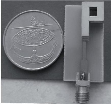
Fig. 8. Photograph of the realized P-shaped dielectric antenna.
