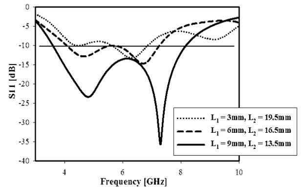
Fig. 7. Simulated  $S_{11}$  of the antenna with different values of  $L_1$  and  $L_2$  ( $W' = 1.4$  mm).
