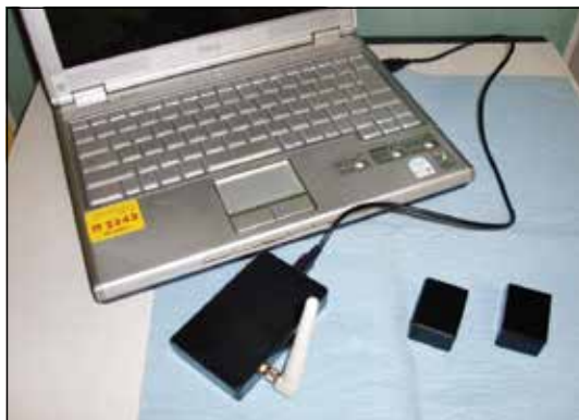
Fig. 3. Triaxial accelerometer for measuring acceleration of the head.
