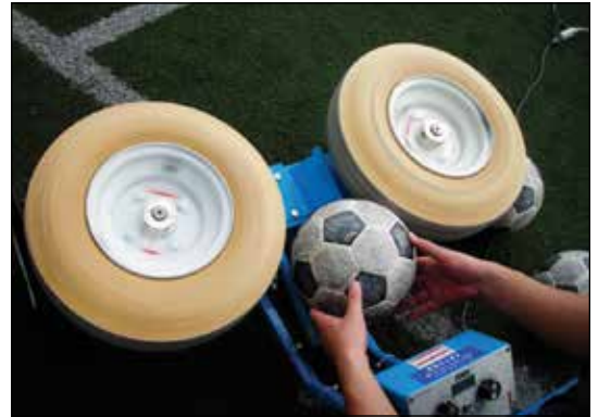
Fig. 2. Soccer machine for duplicating passes.
