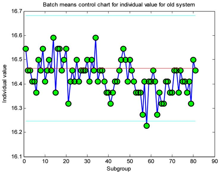
Fig. 11 – Batch means control chart for individual values for old system (second measurements).
