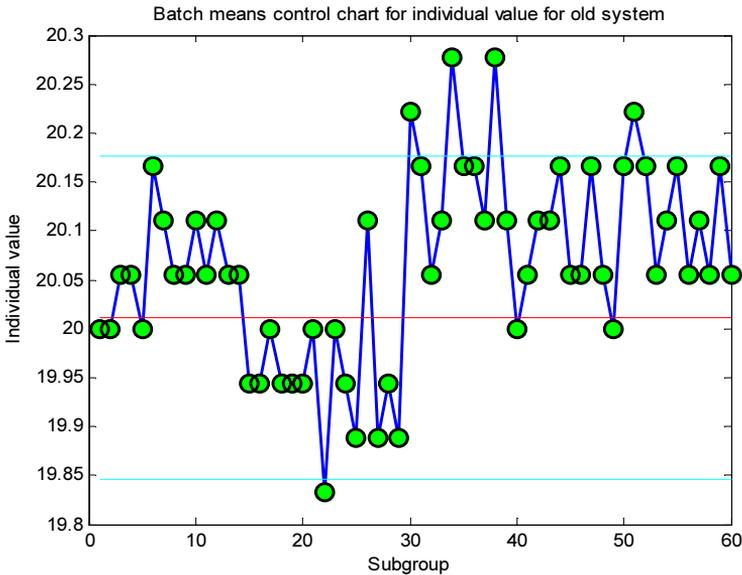
**Fig. 6** – *Batch means control chart for individual values for old system (first measurements).*
