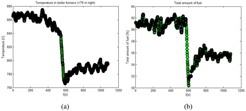
**Fig. 8** – (a) Change of temperature in boiler furnace (+79 m right) for first measurements (b) Time dependency for total amount of fuel for first measurements.
