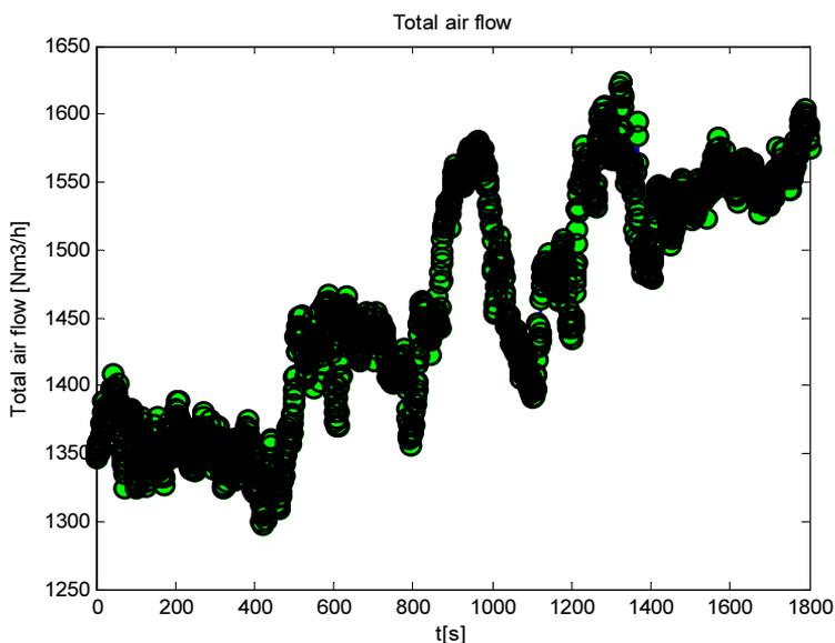
Fig. 13 – Time change of total air flow for second measurements.
