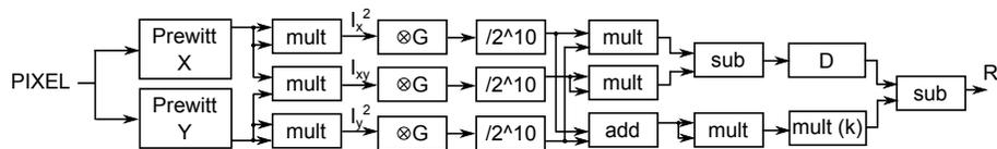
Fig. 6. Scheme of the Harris-Stephens corner detector
