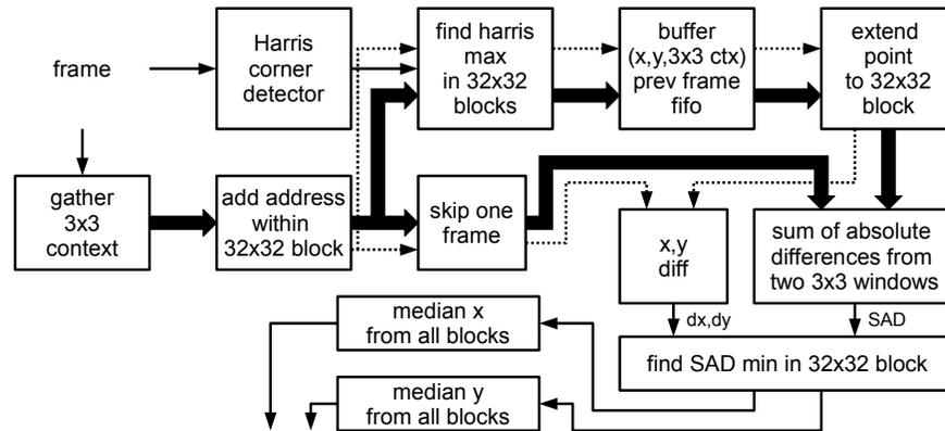
**Fig. 5.** Scheme of the block matching based displacement vector computation module.
