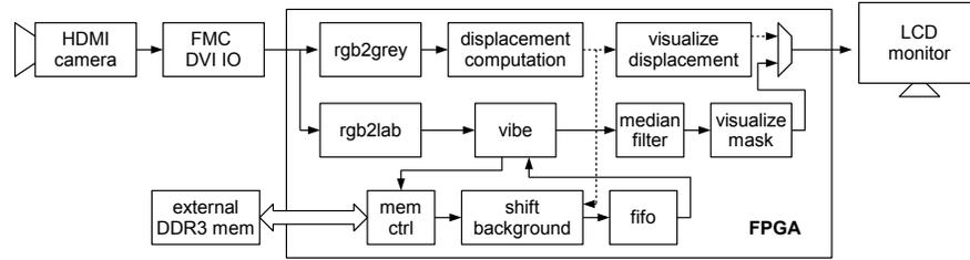
**Fig. 4.** Block diagram of the designed hardware video stream processing system.
