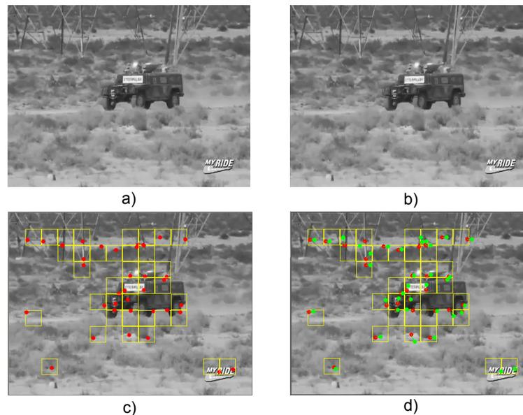
**Fig. 1.** Example of the proposed motion estimation method. a) current frame, b) previous frame, c) result of corner detection in  $32 \times 32$  context – red dots detected corners, d) result of sparse optical flow; previous location (green) and current location (red). The estimated displacement –  $[0, -3]$ . Image sequence from an old DARPA challenge (video available on-line).
