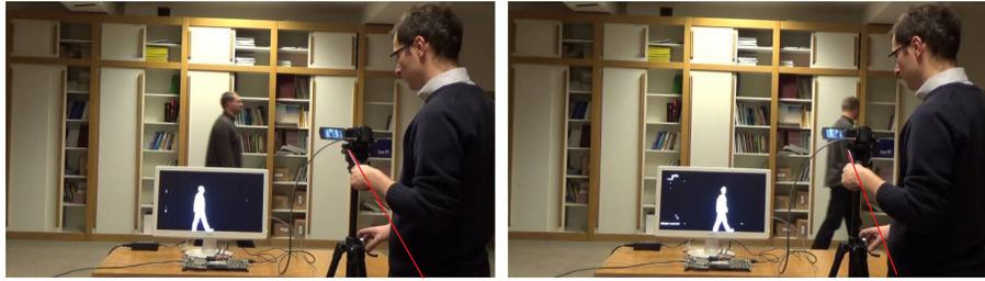
**Fig. 8.** Working system. The operator rotates the HDMI camera, so that the moving person (in the background) is always located in the centre of the image (the overlaid red line indicates the camera direction). The foreground mask (segmentation result) is displayed on the LCD screen. The FPGA development board is visible in front of the LCD.
