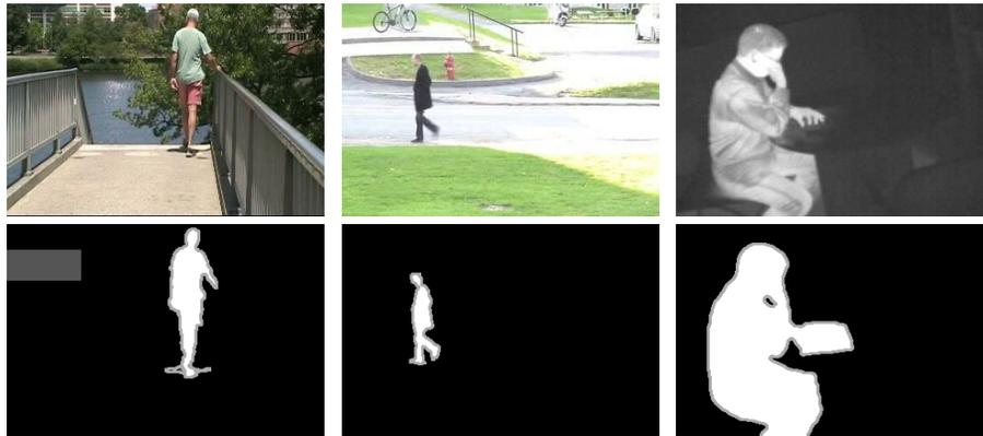
**Fig. 2.** Sample test images from the `changedetection.net` database. Upper row – input images, bottom row column – groundtruth. First column – *overpass* sequence (movement in background), second column – *pedestrians*, third column – *library* (thermal image).
