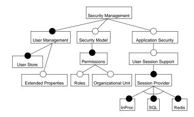
Fig. 5. The feature diagram of the security management subsystem.
