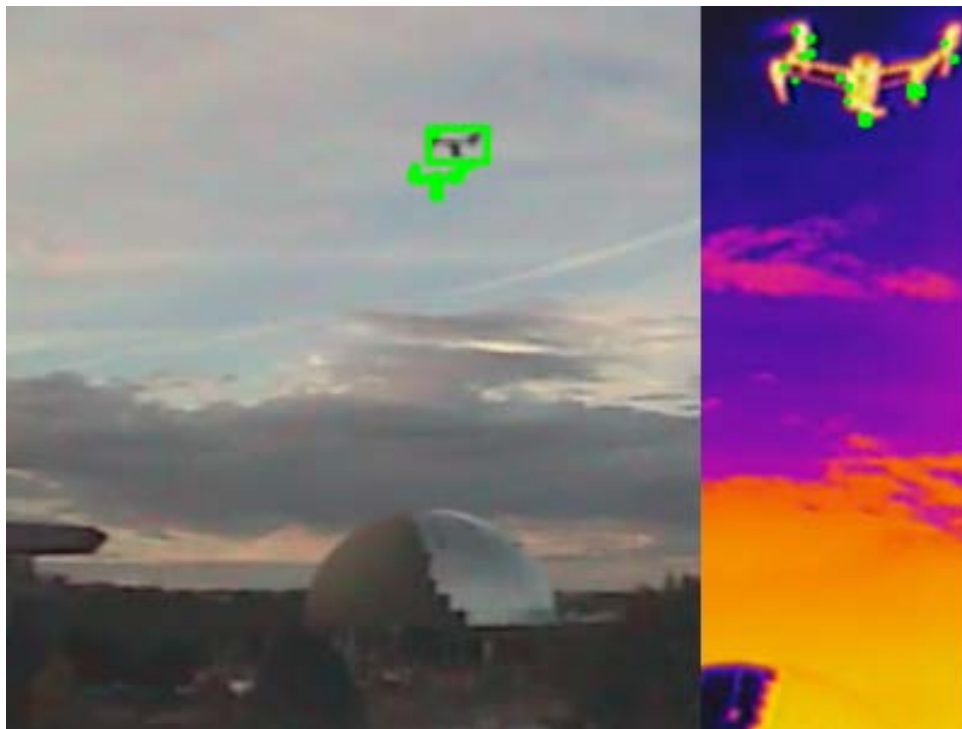
Figure 13. – DJI Inspire Drone Observed by LWIR and Visible band with SDMSI
