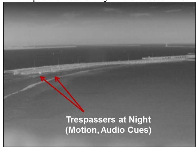
Figure 7. – Trespassers Detected by Audio Cues and LWIR Motion
