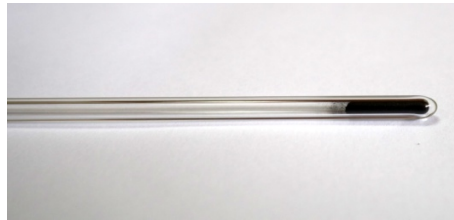
Figure 7. The model eumelanin – DOPA-melanin in the glass tube with diameter of 3 mm for EPR measurements.
