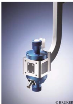
Figure 4. The resonance cavity of CW-EPR spectrometer of Bruker BioSpin GmbH.
