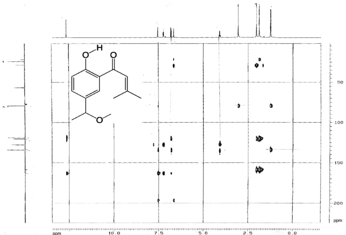
Figure S3. HMBC NMR spectrum ( $\text{CDCl}_3$ ) of compound 1.
