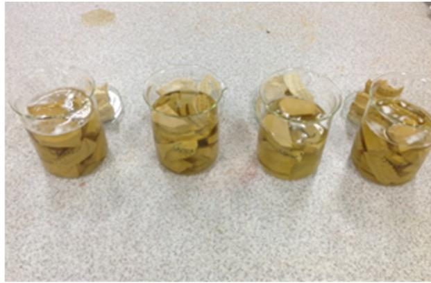
Figure 1: Inoculation of stone casts with suspension of *Bacillus subtilis*
