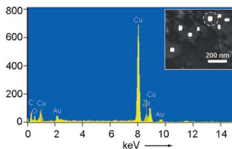
**Figure 3.** EDX spectrum of an asymmetrically modified graphene sheet with ZnO and Au NPs attached to two opposite surfaces. Inset: the corresponding STEM image (the EDX analysis area is indicated by a white circle). Note that the Cu signal comes from the copper TEM grid used in this study.
