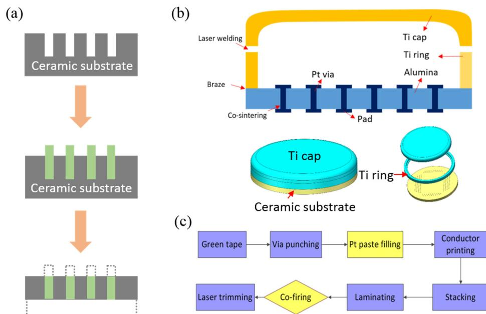
**Figure 2.** (a) Illustration of the package fabrication process described by a patent from Second Sight; (b) the cross-sectional (top) and 3D illustration (bottom) of implantable body for retinal implant with 100+ channel, and (c) the major process flow for platinum/alumina composite substrate in our group.
