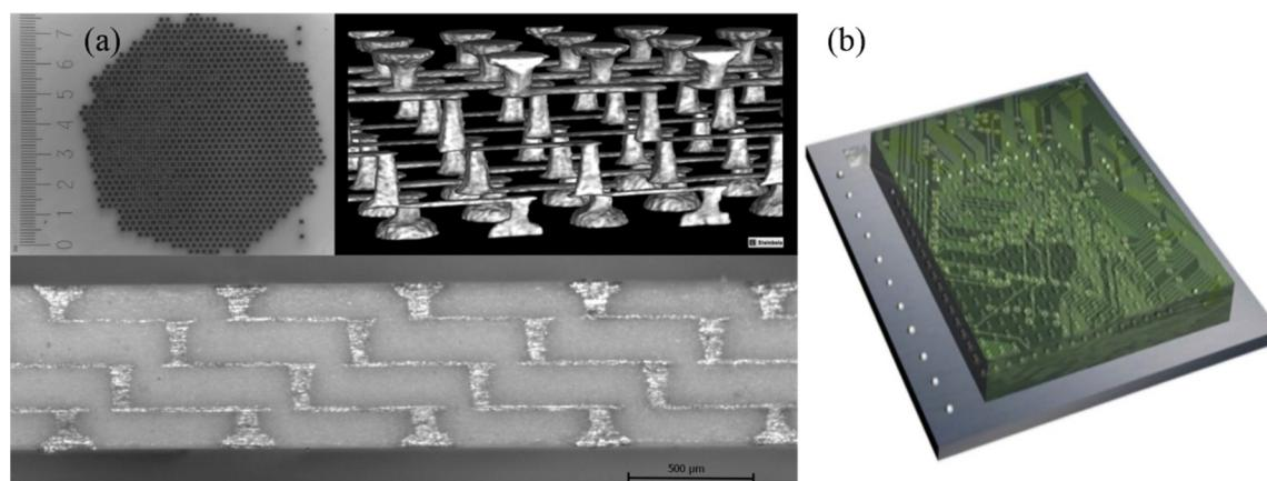
**Figure 3.** (a) The high-density electrode array and corresponding cross-section of hermetic feedthroughs produced with four layers, Reproduced with permission from [44], published by Wiley Online Library, 2014; (b) illustration of a high-density array of diamond feedthrough and electrode with 256 channels, Reproduced with permission from [25], published by Elsevier, 2014.
