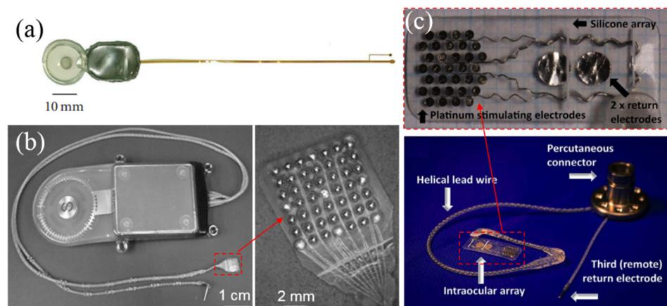
**Figure 8.** (a) A suprechoroidal implant for transretinal stimulation [70]; (b) the supra-choroidal-transretinal stimulation (STS) implant including the suprachoroidal stimulating array and the remote return electrode [77]; (c) the Bionic Vision Australia (BVA) implant with 1 remote return and 2 other return electrodes on the suprachoroidal array [15]. Reproduced from the mentioned references with permission from the related journals.
