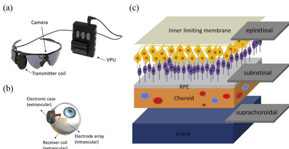
**Figure 1.** (a) External and (b) implant part of the Argus II system [7]; (c) illustration of the implantation sites of the visual cortex, epiretinal, subretinal, and supra-choroidal prostheses [7]. Reproduced with permission from [7], published by Elsevier, 2016.
