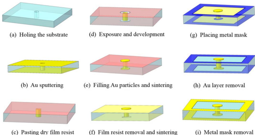
**Figure 4.** Fabrication process of the base wafer: (a) Holing the substrate, (b) Au sputtering, (c) pasting dry film resist, (d) exposure and development, (e) filling Au particles and sintering, (f) film resist removal and sintering, (g) placing metal mask, (h) Au layer removal, and (i) metal mask removal. Reproduced with permission from [46], published by IOPScience, 2016.
