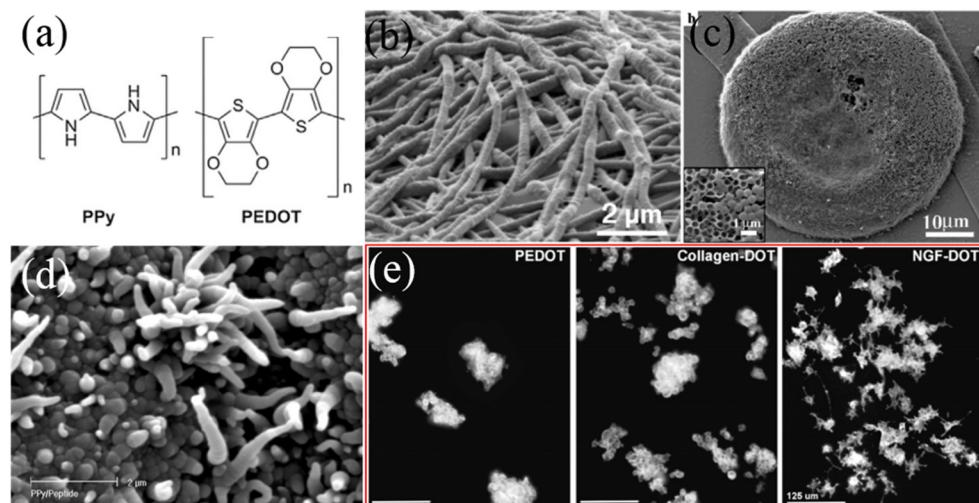
**Figure 10.** (a) Chemical structures of PPy and PEDOT [108]; (b) SEM image of PEDOT coating [109]; (c) SEM image of PEDOT obtained using polystyrene as template [105]; (d) SEM image of PEDOT/DCDPGYIGSR composite coating [106]; (e) Neurotrophic factor combined with PEDOT promoted the growth of neural cells [107]. Reproduced from the mentioned references with permission from the related journals.
