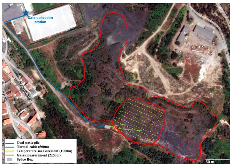
**Figure 3.** General view of the active combustion area in S. Pedro da Cova waste pile and schematic representation of the optical fiber system installation in the field (base map source: Google Earth ©2016 Google Image Landsat Data SIO, National Oceanic and Atmospheric Administration (NOAA), U.S. Navy, National Geospatial-Intelligence Agency (NGA), General Bathymetric Chart of the Oceans (GEBCO)).
