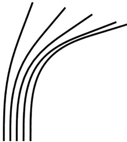
Figure 05. Variations from the same parametric parent. Developed T-Section flanges of the hoops.
