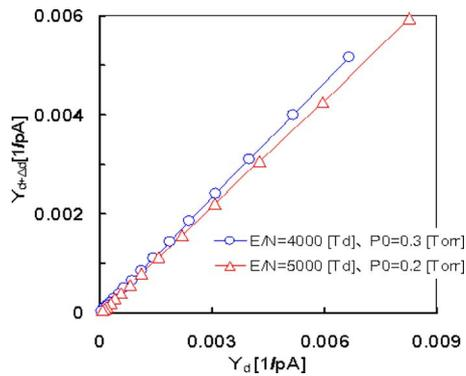
FIG. 5. (Color online) The Gosses plots for the SST experiment with  $\text{CF}_3\text{I}$  at  $E/N=4000$  and  $5000$  Td. Here,  $P_0$  (pressure at  $0^\circ\text{C}$ ) is  $0.3$  Torr and  $\Delta d$  is  $0.03$  cm at  $E/N=4000$  Td, and  $0.2$  Torr and  $0.05$  cm at  $E/N=5000$  Td.
