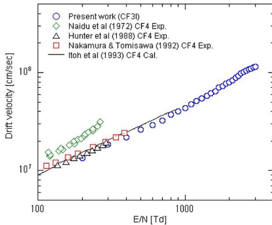
FIG. 1. (Color online) Comparison of the drift velocity. The point in the present work represents the mean arrival-time drift velocity  $W_m$ . In the figure legend, Exp. denotes the experimental result and Cal. the calculated result.
