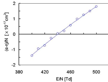
FIG. 3. (Color online) The effective first ionization coefficient,  $\bar{\alpha}/N=(\alpha-\eta)/N$ , in a low  $E/N$  region.
