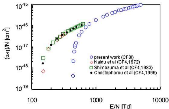
FIG. 2. (Color online) Comparison of the effective first ionization coefficient,  $\bar{\alpha}/N=(\alpha-\eta)/N$ . The data by Christophorou *et al.* (Ref. 2) ( $\text{CF}_4$ ) are recommended values.
