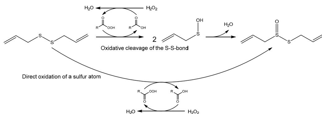
**Scheme 1.** Alliin synthesis from diallyl-disulfide (DADS) through oxidation by a peracid generated with  $\text{H}_2\text{O}_2$  in the reaction mixture. The organic acid serves as an intermediate catalyst.
