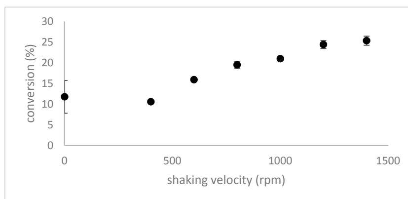
**Figure 3.** The effect of shaking velocity on the reaction rate. Micro-scale reactions using a pre-incubated mixture of H<sub>2</sub>O<sub>2</sub> and formic acid (the reagent mix was stored two weeks at 4 °C) and shaken at various speeds at 0 °C to mix the reactants. Reactions were stopped after 5 min. The maximum reaction rate was achieved by 1200 rpm and statistical analysis according to the Holm-Sidak method showed no significant difference between the rates at 1200 rpm and 1400 rpm.
