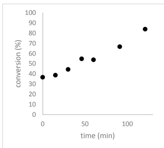
**Figure 5.** Effect of allowing 3 h at  $0^\circ\text{C}$  for the preformation of performic acid on the rate of conversion of DADS to allicin.  $\text{H}_2\text{O}_2$  and formic acid were mixed according to the micro-scale reaction procedure and incubated on ice for 3 h before DADS was added. The reactions were stopped with methanol, separated by HPLC and quantified with a UV detector at 254 nm.
