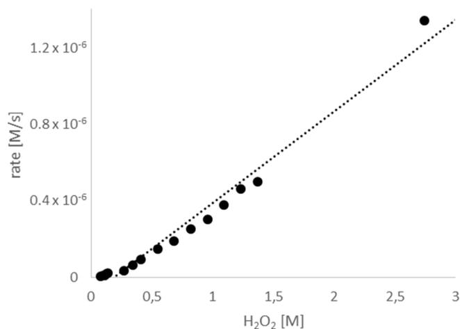
**Figure 4.** The rate of allicin formation in relation to the  $\text{H}_2\text{O}_2$  concentration. Micro-scale reactions were performed with varying  $\text{H}_2\text{O}_2$  concentrations. The reactions were stopped after 30 min, when turnover of  $\text{H}_2\text{O}_2$  was between 14% (start conc. 2.74 M) and 0.9% (start conc. 0.082 M), the linear progression indicates that neither  $\text{H}_2\text{O}_2$  nor DADS were limiting in the reaction.
