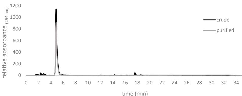
**Figure 9.** Chromatograms of crude allicin after synthesis using formic acid as a catalyst and rotary evaporation and afterwards purification by silica gel chromatography. The crude product contained impurities with retention times of about 2 min and 18 min, respectively, whilst the purified product showed >98% purity. Representative traces of our repeated routine syntheses are shown.
