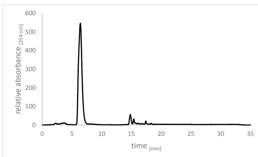
**Figure 8.** Chromatogram of crude alliin after synthesis using pre-formed performic acid. The reaction was extracted with dichloromethane (DCM) and the solvent was removed by rotary evaporation. The crude product already showed good purity.
