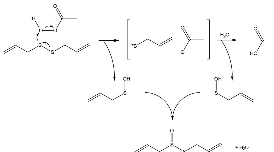
**Scheme 3.** The oxidation of disulfides proceeds via the formation of an allyl cation and an allylsulfenic acid in the first step. In a second step the allyl cation reacts with water to form a second allylsulfenic acid. The resulting sulfenic acids condense in a third step to form allicin.
