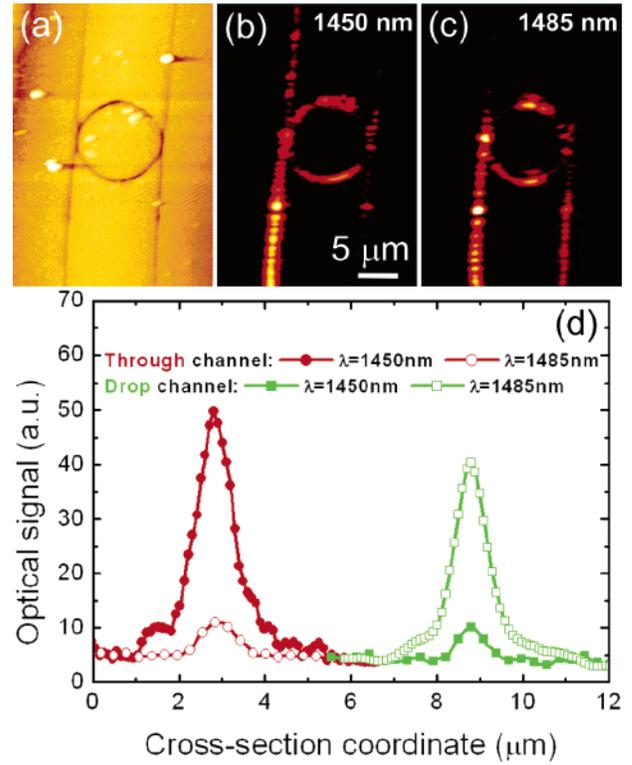
**Figure 2.** Pseudocolor (a) topographical and (b, c) near-field optical images ( $25 \times 35 \mu\text{m}^2$ ) obtained with the investigated WRR-ADM at  $\lambda \approx$  (b) 1450 and (c) 1485 nm. (d) Normalized cross sections obtained from the optical images shown in (b) and (c) for two different output (through and drop) channels with the signal being normalized to be at the same level in the input channel.
