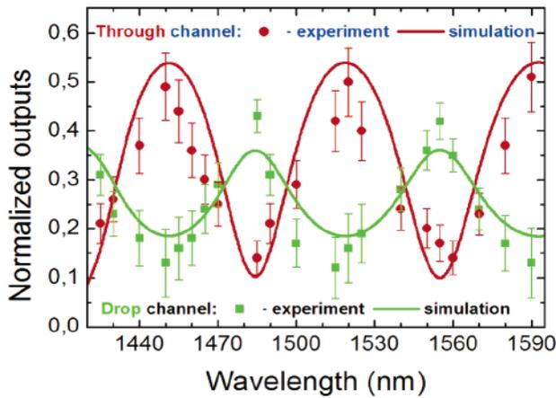
**Figure 3.** WRR-ADM transmission spectra obtained for the through and drop channels along with the fitted curves corresponding to the modeled WRR-ADM response. The output-to-input ratio obtained by using average (along 10 lines) cross sections of near-field optical images (similar to that shown in Figure 2) for both channels. The error bars are estimated from the maximum variation in the ratio when placing the averaging windows at different positions along the input and output channels.
