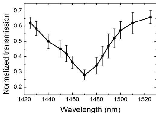
**Figure 5.** BGF transmission spectra representing the output-to-input ratio obtained by using average (along 10 lines) cross sections of near-field optical images (similar to that shown in Figure 4) taken perpendicular to the CPP propagation direction before and after the BGF. The error bars are estimated from the maximum variation in the ratio when placing the averaging windows at different positions along the groove regions (before and after the grating).
