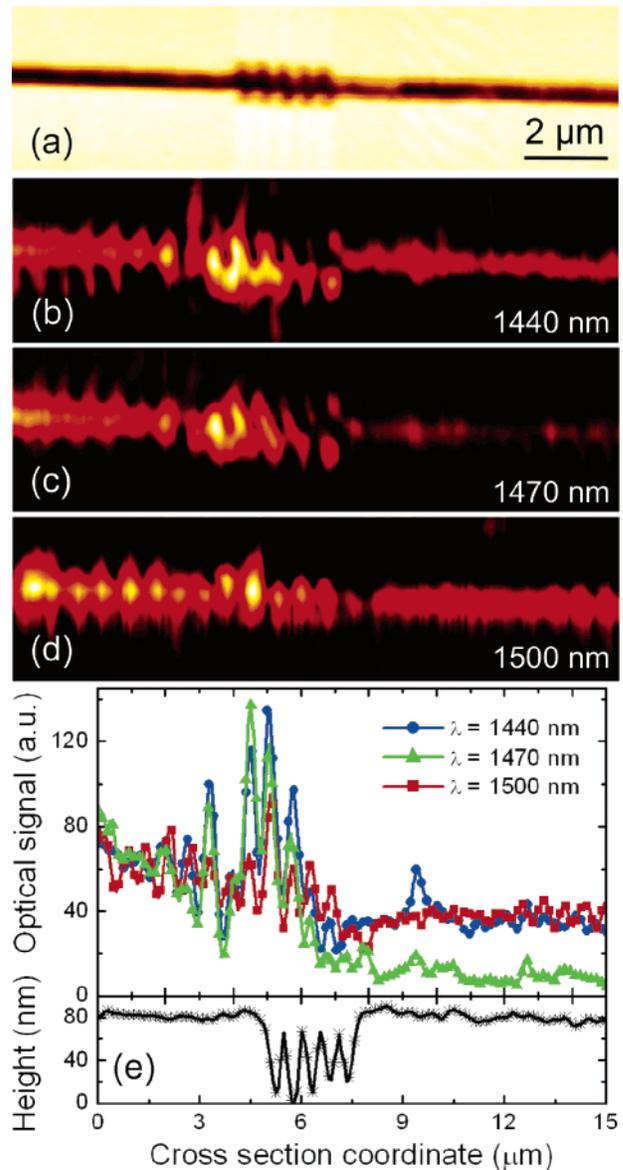
**Figure 4.** Pseudocolor (a) topographical and (b–d) near-field optical images ( $15 \times 4 \mu\text{m}^2$ ) obtained with the investigated BGF at  $\lambda \cong$  (b) 1440, (c) 1470 nm, and (d) 1500 nm. (e) Corresponding cross sections (averaged along 10 lines along the CPP propagation direction) of the topographical (stars) and near-field optical images (filled circles, triangles, and squares) shown in (a–d), respectively.
