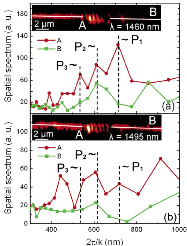
**Figure 6.** Spatial-frequency spectra obtained with near-field optical images (shown in the insets) straight regions of the groove before and after (along the lines marked with A and B) the BGF at  $\lambda \cong$  (a) 1460 and (b) 1495 nm. Positions of the main peaks dominating the spectrum are indicated with dashed lines. The size of the inset optical image is  $20 \times 4 \mu\text{m}^2$ .
