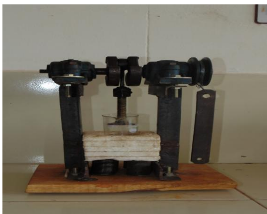
Figure 1. Schematic diagram of chewing chamber of In-vitro chewing apparatus
