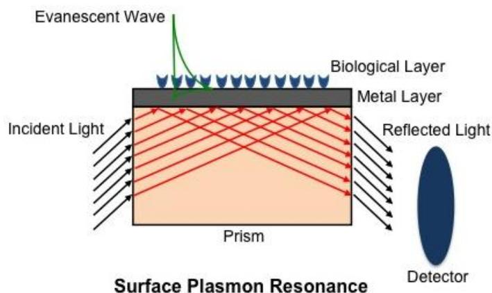
**Figure 2.** Detection of binding events for SPR and RM. As analyte begins to flow over the sensing layer and binds to substrate, the angle of reflectivity that satisfies the resonance condition will change accordingly until it reaches saturation and all the binding sites have been occupied. The dissociation of analyte from the substrate causes the angle of the detector to return back to baseline once all the analyte has been completely removed.
