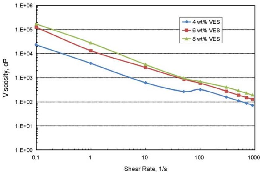
Fig. 2. Temperature: 190°F; HCl concentration: 15 wt%; surfactant concentration: 4 wt%, 6 wt% and 8 wt%; hydrolysis time: 1 hour.
