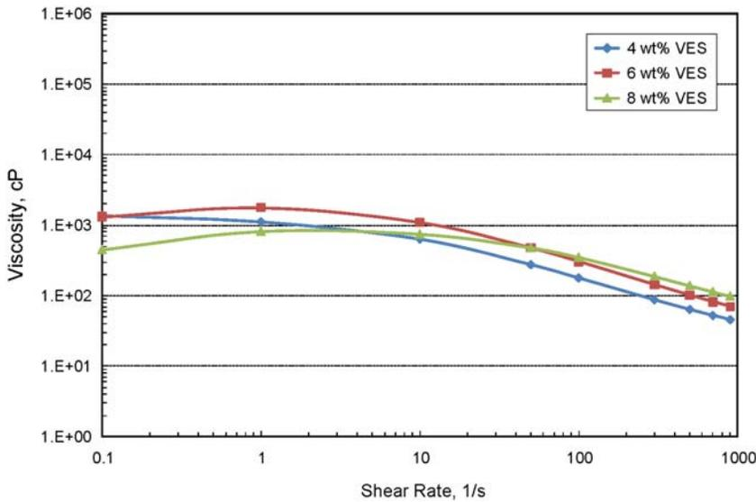
Fig. 1. HCl concentration: 15 wt%; surfactant concentration: 4. wt%, 6 wt% and 8 wt%; hydrolysis time: 0 hour (no hydrolysis).
