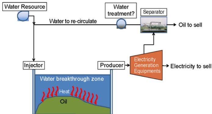
Fig. 1. Heat recovery scheme for electric power generation.
