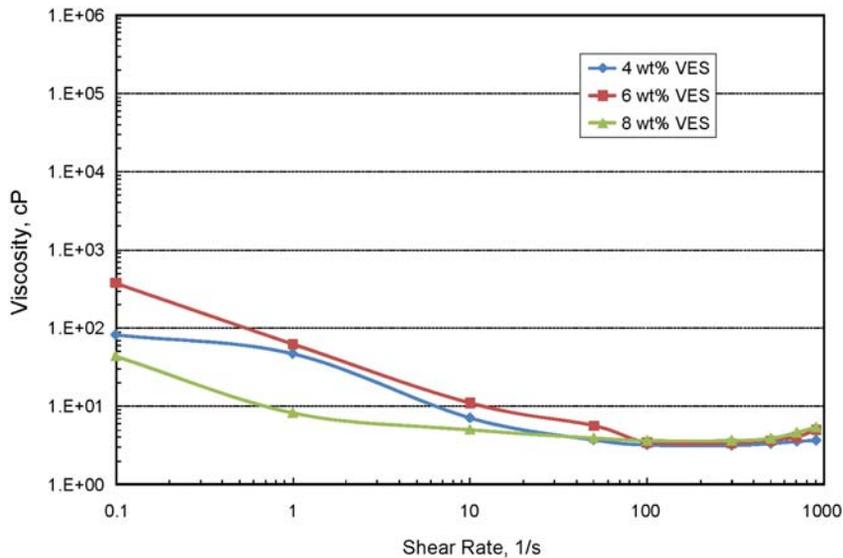
Fig. 3. Temperature: 190°F; HCl concentration: 15 wt%; surfactant concentration: 4 wt%, 6 wt% and 8 wt%; hydrolysis time: 6 hours.
