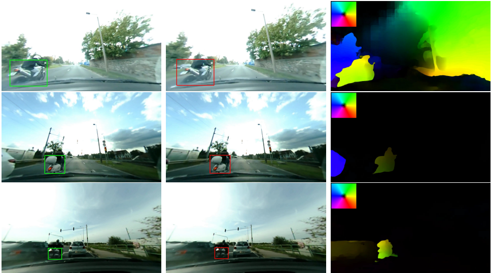
FIGURE 5. Complementing Yolo object detection by optical flow (OF). Three instances are shown in rows. The columns from left to right are: current frame with detected Yolo bounding box, next frame with predicted bounding box, OF from current to next frame visualized. The square represents color coding of OF.
