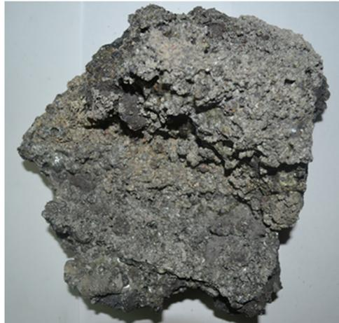
**Figure 1.** A large chunk of palm oil clinker (POC).
