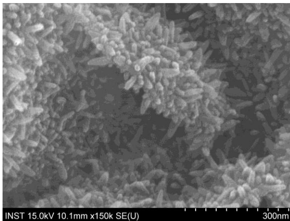
Fig. S2. High resolution SEM image of SnO 2 nanowall electrode showing full coverage of TiO 2 nanoneedles.
