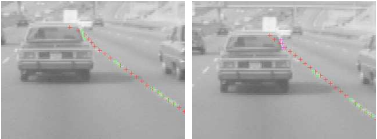
Figure 11: Estimated parameters and zoom showing the feature points (green) and the fitted lane markers (red). Left: all the feature points are used. Right: the spurious feature points (purple) are removed using the residual disparity with respect to the ground plane
