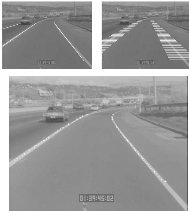
Figure 9: The initialization of the algorithm is done by detection of portions of straight lines of common orientation (top left). Within the search zone predicted (top right), a precise localization of line markers points is performed (bottom).
