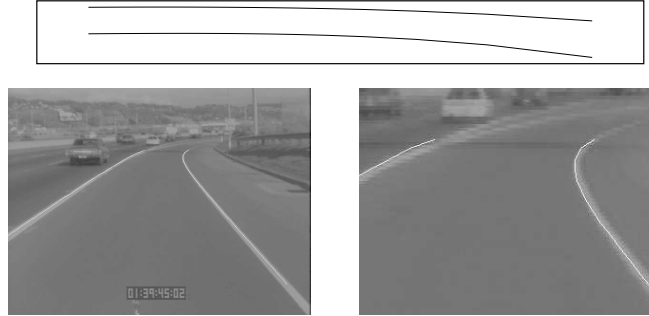
Figure 10: Estimated parameters, top view, and reprojected view of the fitted clothoids. The zoom shows that the fit is quite precise, in spite of the large distance and curvature variation.
