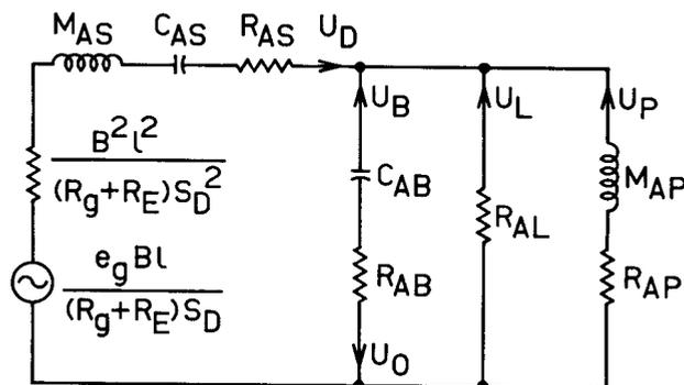
Fig. 1. Acoustical analogous circuit of vented-box loudspeaker system.
