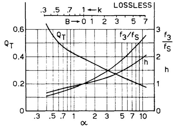
Fig. 6. Alignment chart for lossless vented-box systems.
