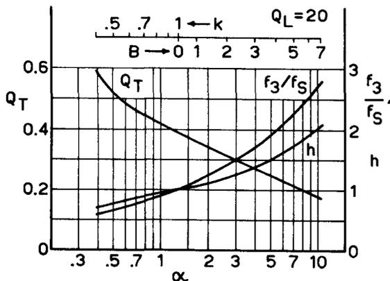
Fig. 9. Alignment chart for vented-box systems with  $Q_B = Q_L = 20$ .
