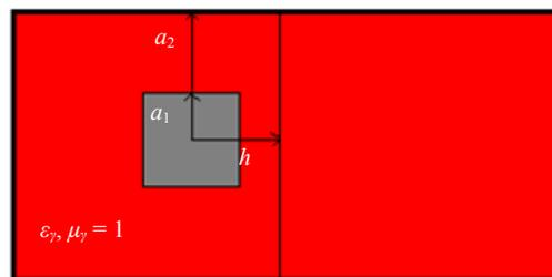
**Figure 2.** Cross section of the rectangular coaxial line with one square inner conductor.
