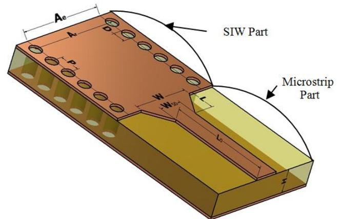
Fig. 1. SIW to Microstrip Transition Design Scheme
