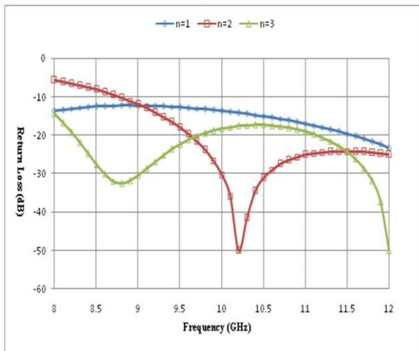
Fig. 4. Return Loss as a function of Taper Length
