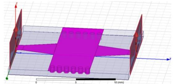
Fig. 3. Back to Back Transitions Simulation Model
