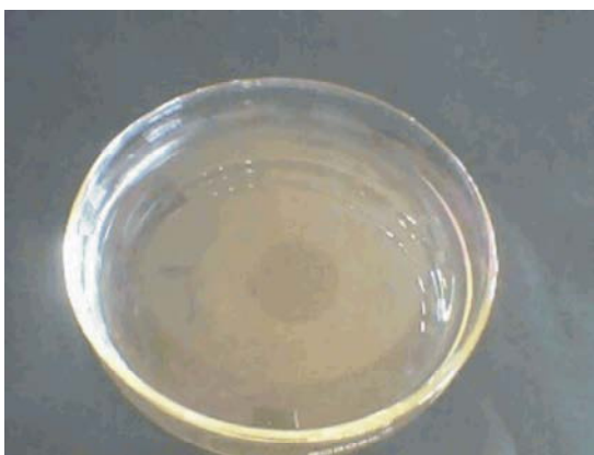
Fig. 2: Zone formation by biosurfactant producing bacteria Pseudomonas aeruginosa in oil spreading technique.
