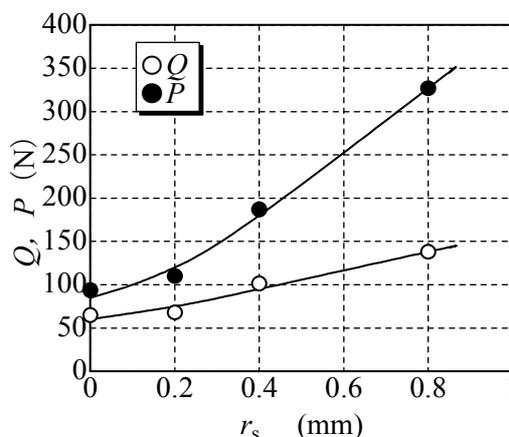
Fig.5 Influence of cutting edge roundness  $r_s$  on cutting forces ( $\alpha = -45^\circ$ ,  $w_f = 0.4\text{mm}$ )
