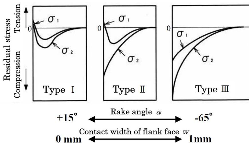
Fig.2 Typical forms of residual stress distribution of cut surface
