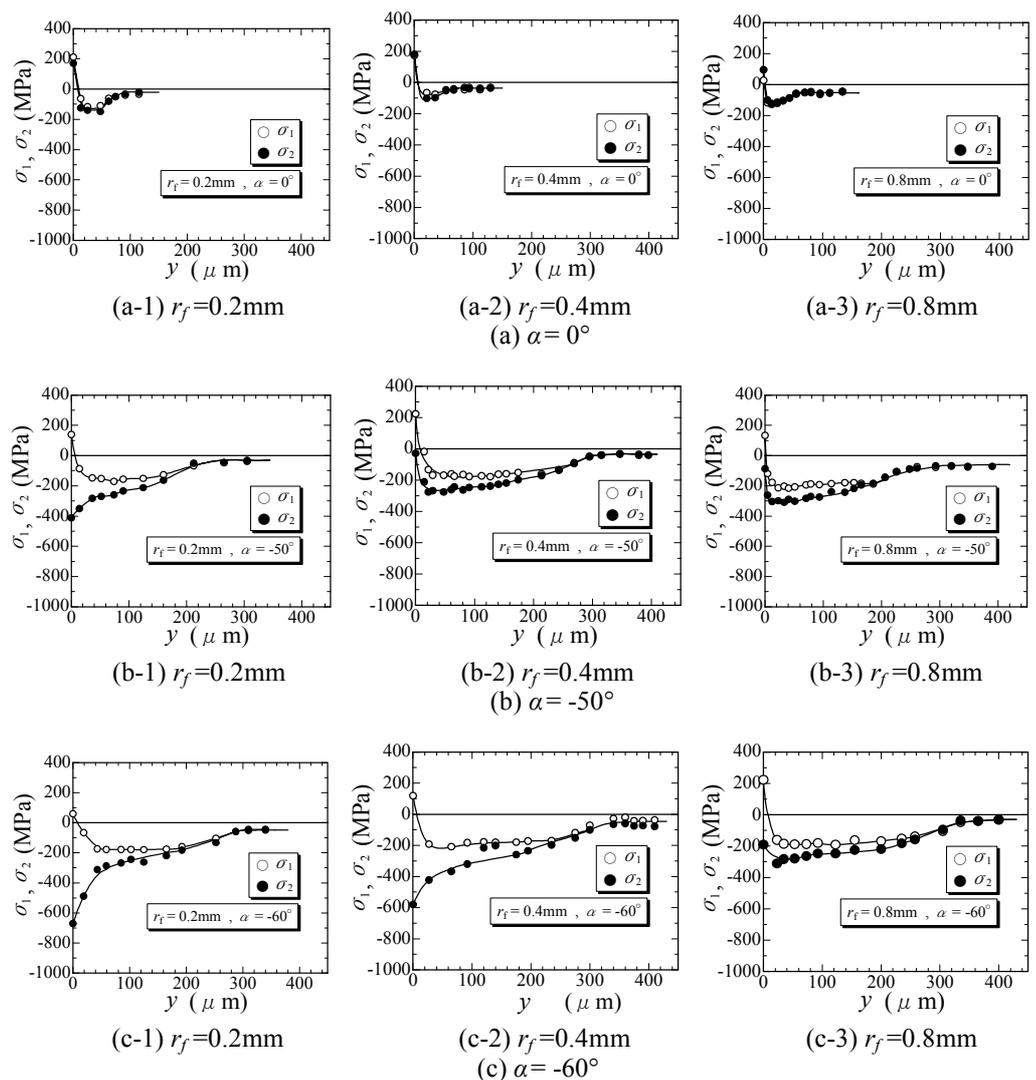
Fig.3 Influence of nose radius  $r_f$  on residual stress distribution
