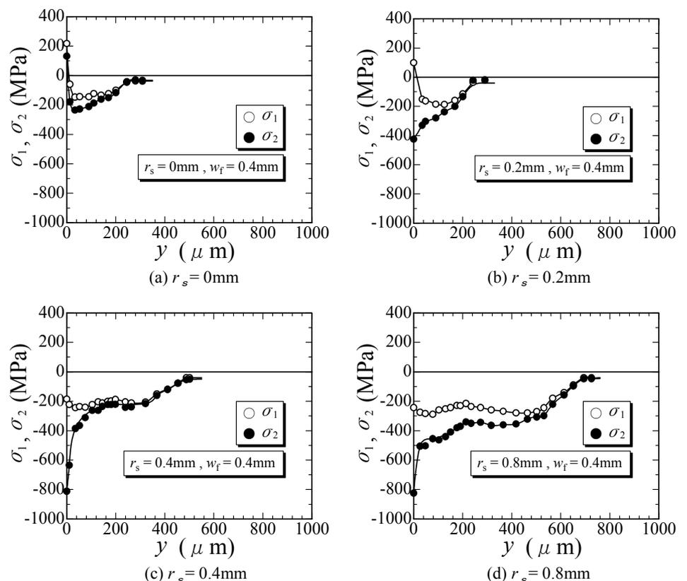
Fig.4 Influence of cutting edge roundness  $r_s$  on residual stress distribution ( $\alpha = -45^\circ$ ,  $w_f = 0.4$  mm)
