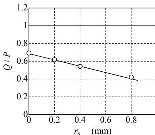
Fig.6 Influence of cutting edge roundness  $r_s$  on cutting force ratio ( $\alpha = -45^\circ$ ,  $w_f = 0.4\text{mm}$ )
