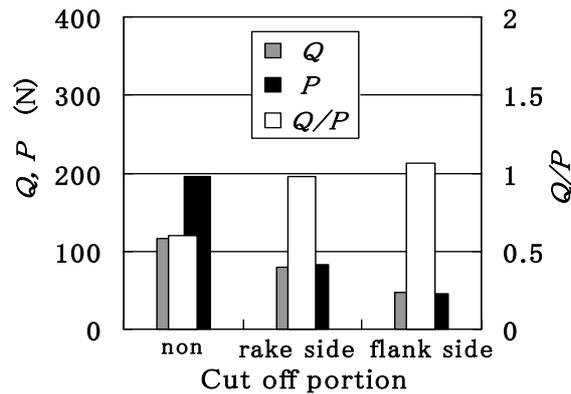
Fig.8 Influence of cut off portion on cutting forces and force ratio
