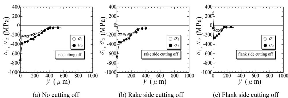
Fig.7 Influence of cut off portion on residual stress distribution
