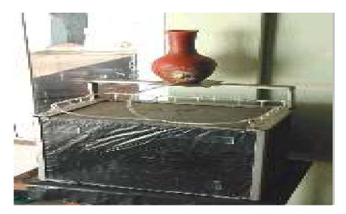
Figure 01: Evaporative cooling unit
