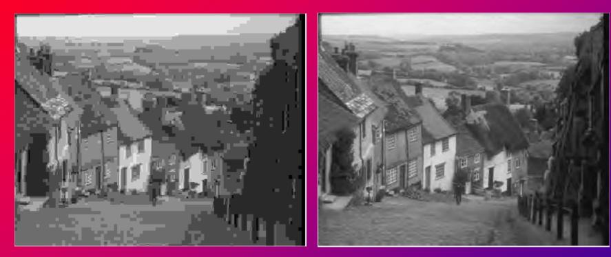
discrete cosine transform based JPEG (CR=64) wavelet transform based JPEG2000 (CR=64)
